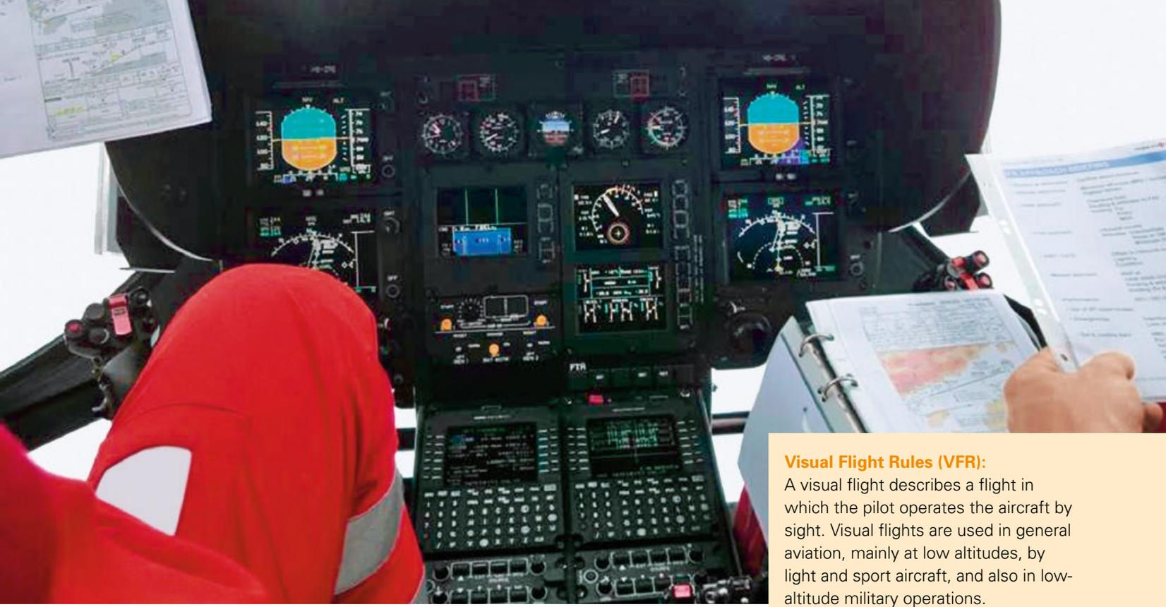
**IFR-compatible cockpit: in 2014, all of Rega's Da Vinci helicopters will be equipped for instrument flights.**
