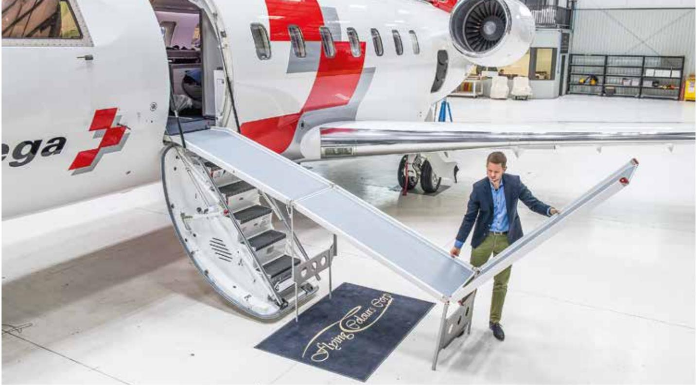
**Improved design: the new ramp makes loading and unloading more comfortable for patients.**
