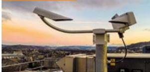
**Precise flight weather data** 60 new or enhanced measuring stations and weather cameras now continually supply Rega's helicopter pilots with up-to-date meteorological information – a key prerequisite for IFR flights.
