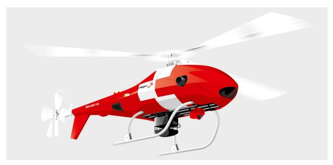
The Rega drone unites cutting-edge technology with Rega's decades of experience in conducting search operations for missing, injured or ill persons. It autonomously scans large search areas and is equipped with various search systems. The Rega drone is deployed when, for example, the rescue helicopter is forced to remain on the ground due to poor visibility.
